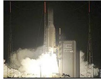
The Ariane 5 ECA is the latest version of the Ariane 5 launcher. It is designed to place payloads weighing up to 9.6 tonnes into geostationary transfer orbit. With its increased capacity Ariane 5 ECA can handle dual launches of very large satellites.
